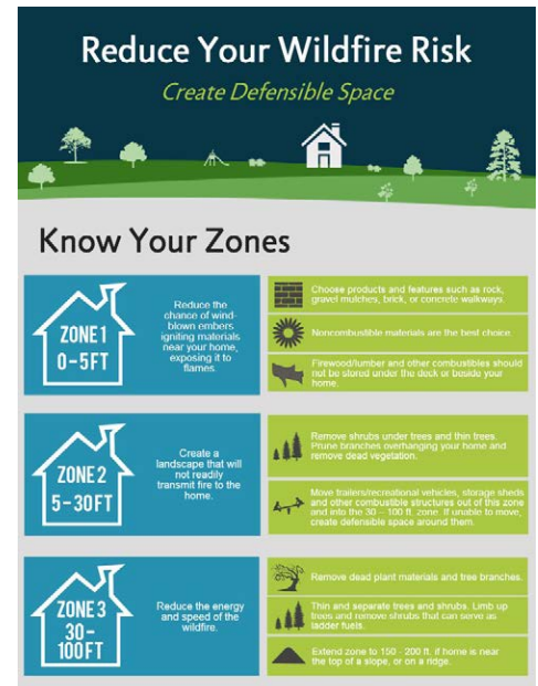
Figure 35. The building components of a home (e.g., roofing and siding), together with the home's surrounding vegetation, are primary factors in whether a home is vulnerable to wildland fire embers. Wildland fire risk can be reduced through the creation of defensible space around the home. Source: Insurance Institute for Building and Home Safety.
