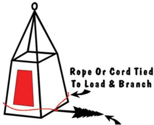
5 Exhibit 11.4 – Rigging a Box-like Load with a Tree Branch as a Tail.
