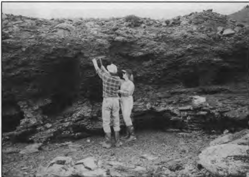
Figure 6. Typical wave-cut terrace in thinly bedded slag that was deposited in the molten phase (sample site 11). This site has fewer secondary minerals forming compared to the other sample sites.
