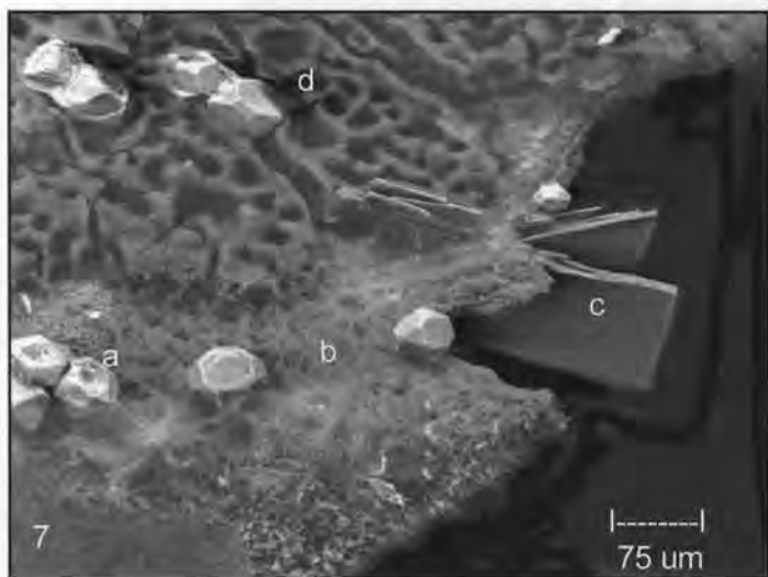
Figure 13. SEM/BSE image of secondary minerals lining a vesicle at site 6: a , undescribed emerald green crystals; b , cottony bluish Cu chloride; c , botallackite; d , Ca sulfate that may be gypsum.
