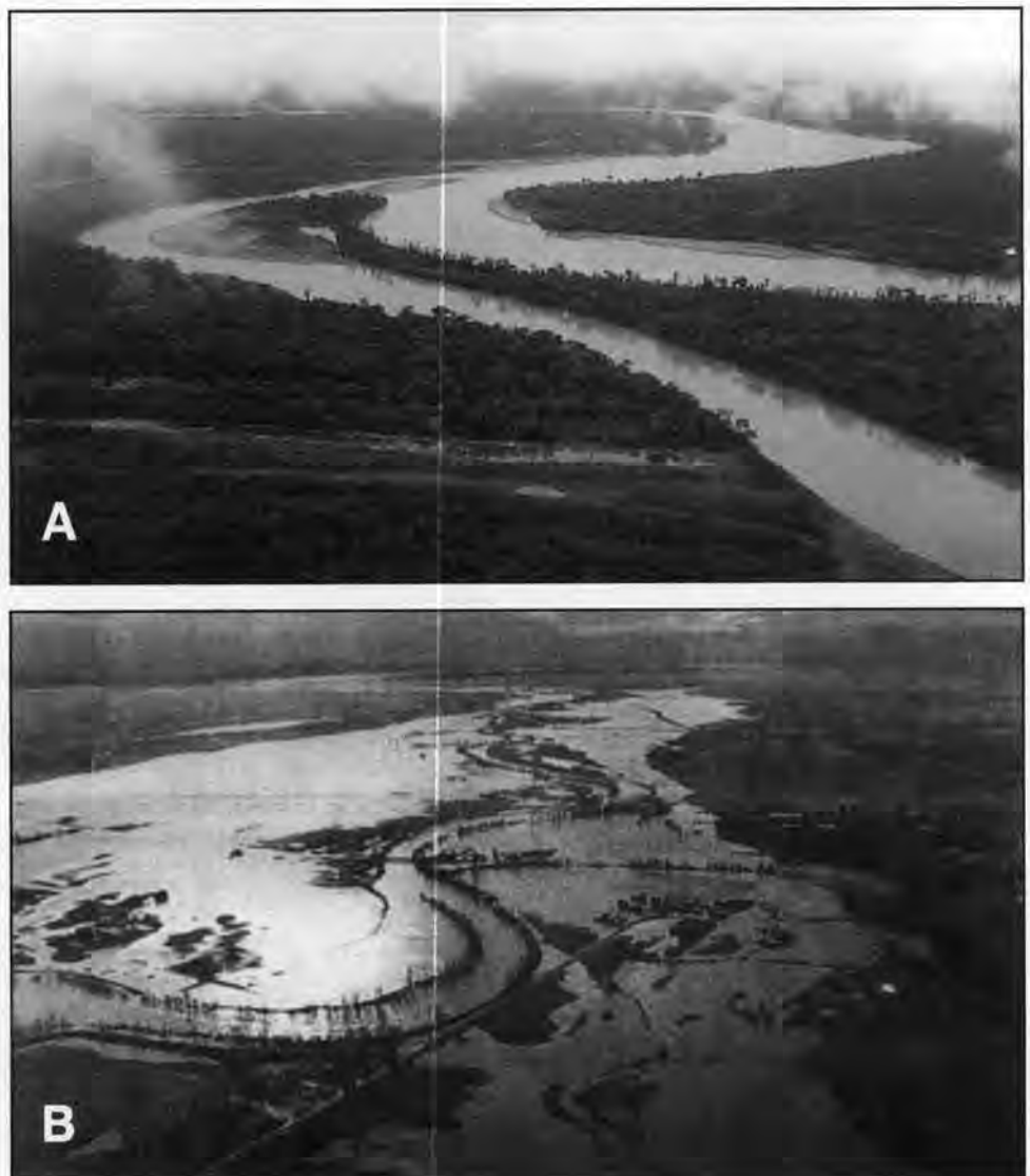
Figure 3. Depositional environments characteristic of modern meandering rivers. A. When flow is normal, sedimentation is limited to deposition of point bars at the inside bends of the channel, where the current is retarded. Higher velocities at the outside of the bend erode the bank, gradually causing the channel to migrate laterally. Modern rivers have been known to shift their channel by as much as several hundred meters per year (Wolman and Leopold, 1957). Although each point bar occupies only a small area, channel migration eventually distributes bar deposits over the entire flood plain, causing them to be the dominant type of sediment. Napo River, an Amazon tributary. Photo by Peter Frey. B. During floods, meandering rivers distribute silt and fine sand over adjacent lowlands in ribbon-like deposits that may be many kilometers in length, but only a few centimeters in thickness. Nooksack River during the December 1995 flood. Photo by Philip A. Dwyer/Bellingham Herald. Used with permission.
